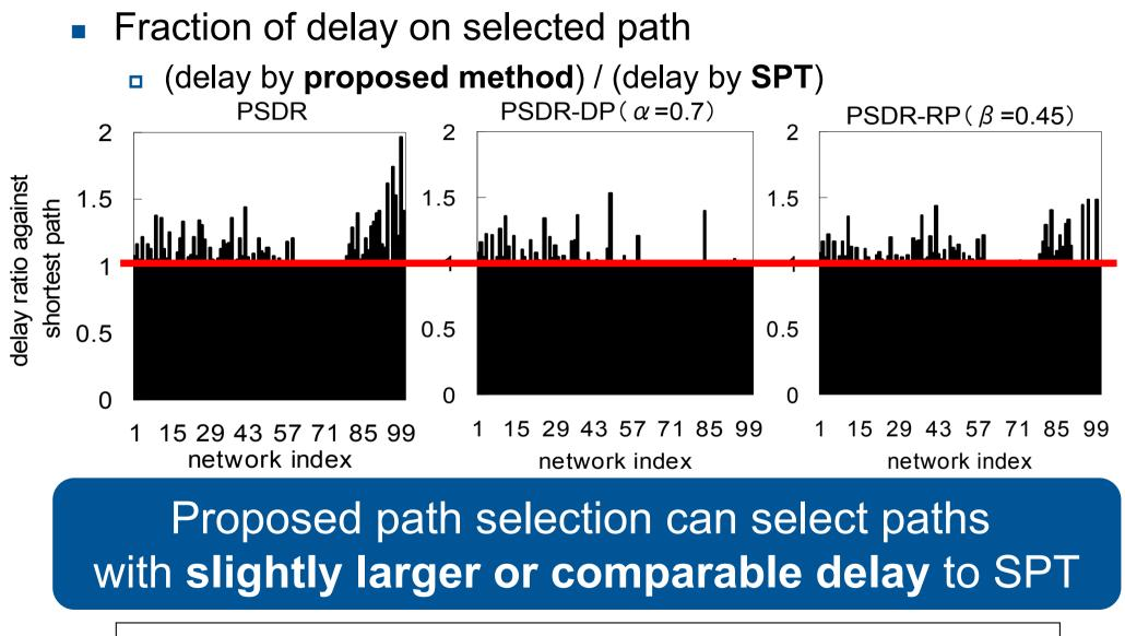
Small delay within allowable delay for live streaming media
