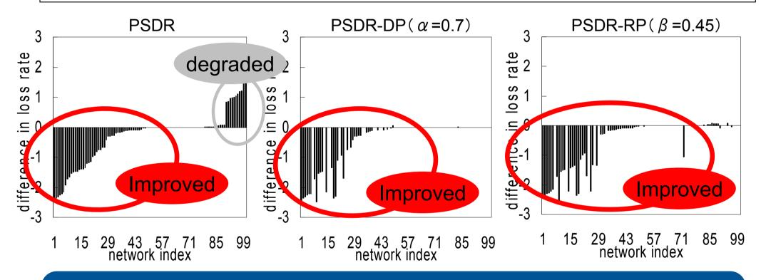
Proposed path selection can select paths that reduce end-to-end loss rate better than SPT
